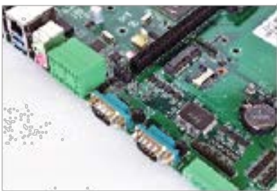
8KV ESD, TVS 600W Surge Protection for COM port
