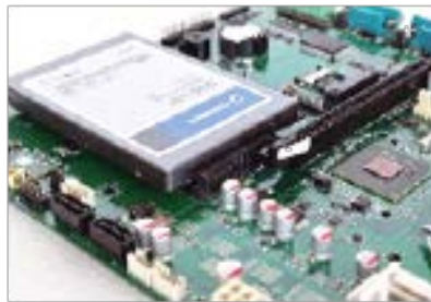
Direct HDD connection No internal cabling
