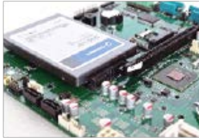
Direct HDD connection No internal cabling
