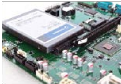
Direct HDD connection No internal cabling
