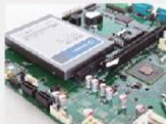
Direct HDD connection No internal cabling
