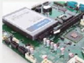
Direct HDD connection No internal cabling
